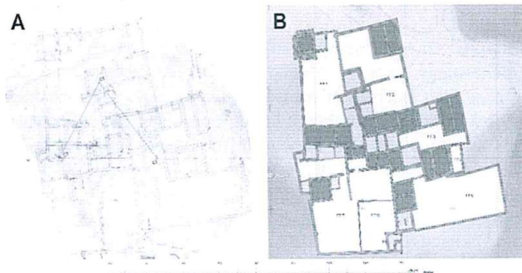
Fig. 5. Topographic survey with the Zeiss BRT 006 tachymeter and the Karti table. A - superimposed Karti table rings with field observations; B – ready to publish drawing of the same area 4 .
